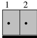
JP2 to JP9 are used to select input voltage range. The JP2 is used to select photo couple input channel 0, and JP3 is used to select photo couple input channel 1 ... etc. When short the jumper, the input voltage range from 0 to 20V, and the active voltage form 3 to 20V. When open the jumper, the input voltage range from 0 to 30V, and the active voltage from 17.6 to 30V.
