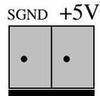
The power of USB 8 channels relay output / photo isolator input card can be supplied from USB, however, if USB can not supply enough power, the external power is need. TB1 is used to input external DC +5V power. Be careful to input DC +5V power.
