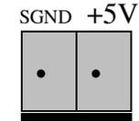
The power of USB 16 channels relay output / photo isolator input card can be supplied from USB, however, if USB can not supply enough power, the external power is need. TB1 is used to input external DC +5V power. Be careful to input DC +5V power.
