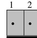
JP2 to JP17 are used to select input voltage range. The JP2 is used to select photo couple input channel 0, and JP3 is used to select photo couple input channel 1 ... etc. When short the jumper, the input voltage range from 0 to 20V, and the active voltage form 4.5 to 20V. When open the jumper, the input voltage range from 0 to 30V, and the active voltage from 18 to 30V.
