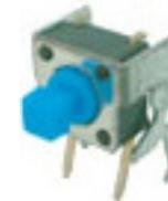
The S1 switch is used to reset 8051, the signal assignments are shown in the following.
