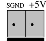
The power of USB 16 channels photo couple input/output card can be supplied from USB, however, if USB can not supply enough power, the external power is need. TB1 is used to input external DC +5V power. Be careful to input DC +5V power.
